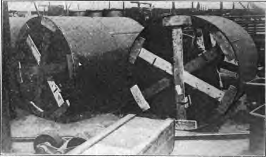
FIG. 144.—Sections of sugar-drier drum, 6 ft. diam. \times 8 ft. long, braced for export shipment.
